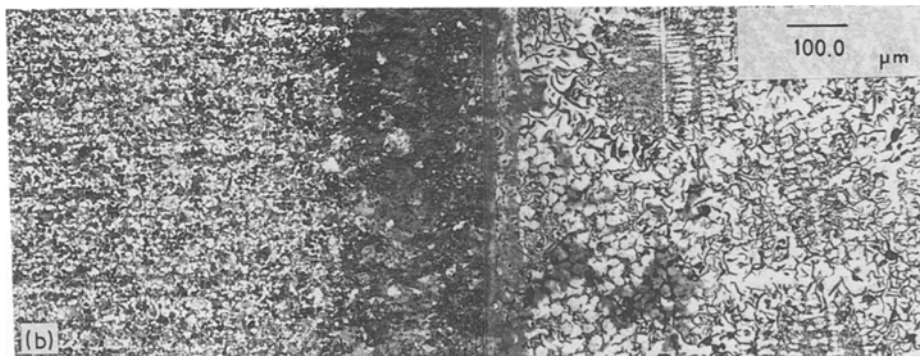
Figure 2 (a) ARMCO iron/cast iron diffusion-bonded joint ( T_b = 880^\circ\text{C} , t_b = 20 \text{ min} , P_s = 4.5 \text{ MPa} ) \times 72 . (b) 0.55% C steel/cast iron diffusion-bonded joint ( T_b = 980^\circ\text{C} , t_b = 10 \text{ min} , P_b = 4.5 \text{ MPa} ) \times 72 .
